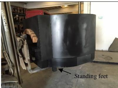
After reaching the installation position, lift the oven up to a working height for the correct positioning on the standing support.
