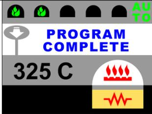
The oven's operating mode upon baking time completion or upon the operator's request, it activates an audible signal during approximately 4 seconds which is followed by a temporary reduction in the deck rotation speed.
