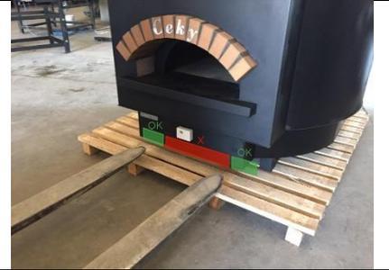
Load the oven's body inserting the forks as shown in the figure (see green rectangles, close to the oven's standing feet).
