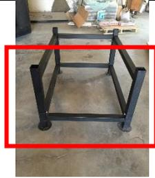
Once the standing support has been mounted, position the structure in the area where the oven will be installed.
