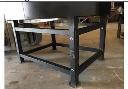
Lower the oven till it lays completely on the standing support's verticals.
